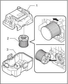
1. Tank cover 2. HEPA filter 3. Tank
