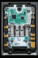
Terminal short-circuit prevention structure. The protection wall is provided between terminals against water and dust.
