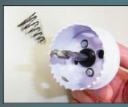
Adjust positions pins and put them into the hole saw
