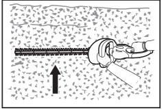
Cut upwards with both hands pull the switch triggers B and C and move it in front of your body.
