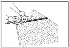
Hold the trimmer with both hands pull the switch trigger A or B and move it in front of your body.
