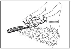
Attaching the chip receiver (accessory) on the tool when trimming the hedge straight can avoid cut off leaves' being thrown away.
