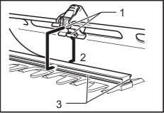
▶ 1. Hooks 2. Fit the hooks into groove 3. Grooves
