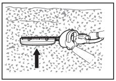
To cut a hedge side evenly, it helps to cut from the bottom upwards.
