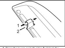
Press the levers on both sides 2. Unlock the hooks
