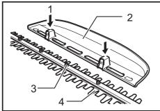
1. Press 2. Chip receiver 3. Nut 4. Shear blade
