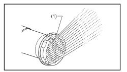
To install the deflector (1), mount the deflector on the top nozzle so that the "I" mark (3) on it is aligned with the "I" mark (4) of the top nozzle (2). Secure the deflector by turning it fully clockwise.
