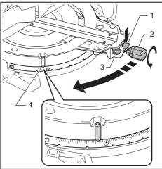
Lock lever 2. Grip 3. Releasing lever 4. Pointer
