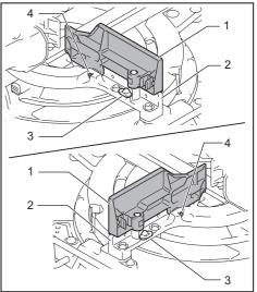
1. Upper fence 2. Lower fence 3. Clamping screw
