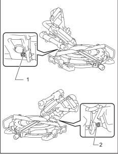
Left 45° adjusting bolt 2. Right 45° adjusting bolt
