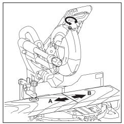
A) When you want to obtain the correct size on the left side of workpiece, shift the laser line to the left of the blade.
