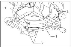
1. Screw on pointer 2. Screws on miter angle scale
