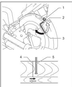
1. Adjusting screw 2. Range adjustment screw
