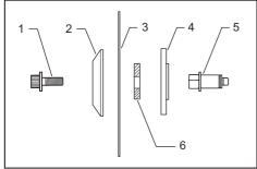
1. Hex socket bolt 2. Outer flange 3. Saw blade
