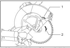
Arrow on the blade case 2. Arrow on the blade
