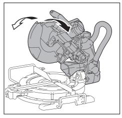
If the pointer does not indicate the  $45^{\circ}$  position, align it with  $45^{\circ}$  position by turning the adjusting bolt on the opposite side of the bevel angle scale.
