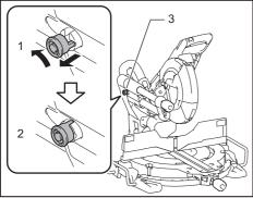
Unlocked position 2. Locked position 3. Stopper pin
