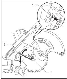
Shaft lock 2. Hex wrench 3. Hex socket bolt (lefthanded) 4. Loosen 5. Tighten
