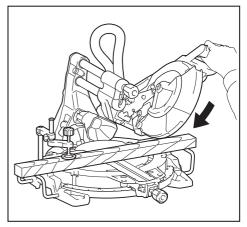
1. Remove the upper fence on the side that you are going to tilt the carriage.
