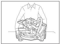
AWARNING: Stopper pin for carriage elevation is for carrying and storage purposes only and not for any cutting operations. The use of the stopper pin for cutting operations may cause unexpected movement of the saw blade resulting in kickback and serious personal injury. **ACAUTION:** Always secure all moving portions before carrying the tool. If portions of the tool move or slide while being carried, loss of control or balance may occur and result in personal injury.
