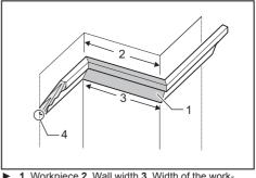
1. Workpiece 2. Wall width 3. Width of the workpiece 4. Wall contact edge
