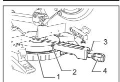
▶ 1. Miter scale 2. Pointer 3. Lock lever 4. Grip
