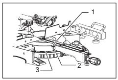
■ 1. Screw 2. Pointer 3. Miter scale
