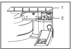
Sliding fence 2. Clamping screw
