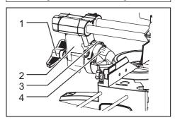
▶ 1. Lever 2. Arm 3. Pointer 4. Bevel scale
