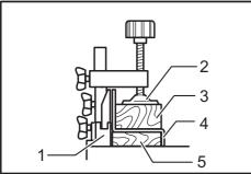
Guide fence 2. Vise 3. Spacer block 4. Aluminum extrusion 5. Spacer block
