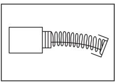
Remove and check the carbon brushes regularly. Replace when they wear down to 3 mm in length. Keep the carbon brushes clean and free to slip in the holders. Both carbon brushes should be replaced at the same time. Use only identical carbon brushes.
