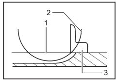
Top surface of turn base 2. Periphery of blade
