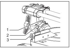
▶ 1. Screw 2. Pointer 3. Bevel scale
