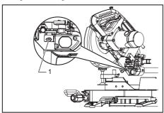
1. Screw holding the laser unit box
