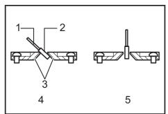
Saw blade 2. Blade teeth 3. Kerf board 4. Left bevel cut 5. Straight cut
