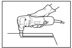
Hold the tool so that the cutting head is at a right angle  $(90^\circ)$  to the workpiece being cut. Move the tool gently in the cutting direction.
