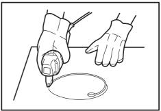
Cutouts can be done by first opening a round hole over 21 mm in diameter which the cutting head can be inserted into.
