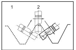
1. From the side view 2. Cutting head should be at a right angle (90°) to cutting surface.
