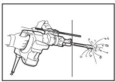
Hold the tool firmly with both hands. Turn the tool on and apply slight pressure on the tool so that the tool will not bounce around, uncontrolled. Pressing very hard on the tool will not increase the efficiency.
