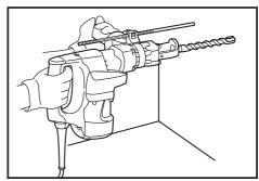
Position the bit at the desired location for the hole, then pull the switch trigger. Do not force the tool. Light pressure gives best results. Keep the tool in position and prevent it from slipping away from the hole.
