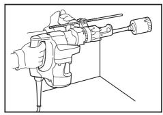
To remove the core bit, hold the adapter with the wrench, insert the rod (optional accessory) into the hole in the core bit and tap with a hammer to unscrew.
