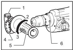
1. Grip base 2. Tighten 3. Loosen 4. Teeth 5. Side grip 6. Protrusion
