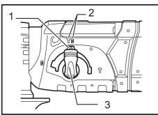
1. Lock button 2. Rotation with hammering 3. Action mode changing knob
