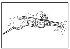
Set the action mode changing knob to the  $\widehat{\mathbb{T}}$  symbol. Hold the tool firmly with both hands. Turn the tool on and apply slight pressure on the tool so that the tool will not bounce around, uncontrolled. Pressing very hard on the tool will not increase the efficiency.
