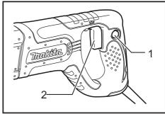
▶ 1. Lock button 2. Switch trigger
