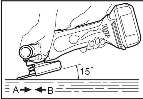
ALWAYS hold the tool firmly with one hand on housing and the other on the side handle. Turn the tool on and then apply the wheel or disc to the workpiece. In general, keep the edge of the wheel or disc at an angle of about 15 degrees to the workpiece surface. During the break-in period with a new wheel, do not work the grinder in the B direction or it will cut into the workpiece. Once the edge of the wheel has been rounded off by use, the wheel may be worked in both A and B direction.
