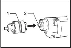
▶ 1. Drill chuck 2. Spindle
