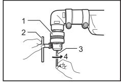
▶ 1. Drill chuck 2. Chuck key 3. Hex wrench 4. Tighten
