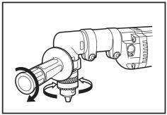
Screw the side grip for the angle attachment on the angle housing. Then tighten the side grip by turning clockwise at the desired position.
