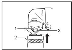
▶ 1. Two faces 2. Drill chuck 3. Spindle
