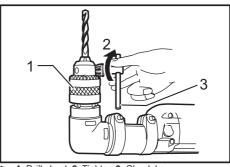
▶ 1. Drill chuck 2. Tighten 3. Chuck key
