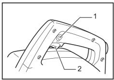
▶ 1. Lock button / Lock-off button 2. Switch trigger
